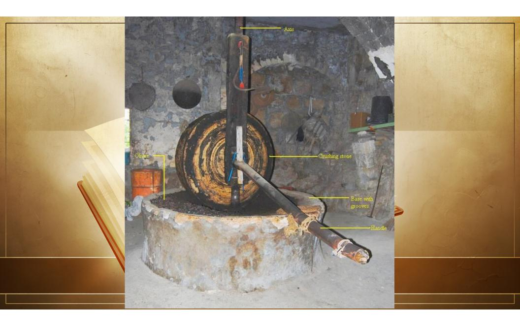
The olive crusher was the stone basin that was used to crush olives into pulp. A donkey pushed on a horizontal beam, which in turn rolled a millstone that crushed ripe olives (placed in a large, round basin) into a pulp.
